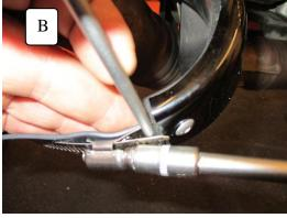
• Remove or loosen the jubilee clip and cut excess off approx 4-5mm from mark (using hack-saw or good quality tin-snips), this will allow the 4-5mm to be tucked between the jubilee clip and the silicon mounting strip to keep things neat, safe and tidy.
